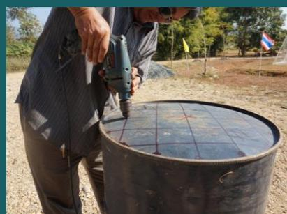
Use the drill with the 1/8" drill bit to drill set holes at every X. Follow up by re-drilling all holes with a 1/2" bit.
